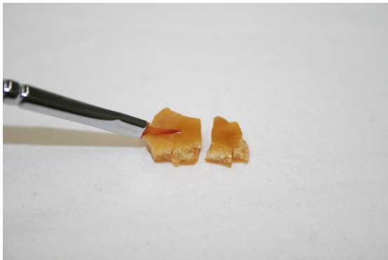
Figure 13. Consolidation of the surfaces and fractured sections of the central ornament fragments of hatstring(22245) with 1% and 3% Plectol D 498 emulsion.
