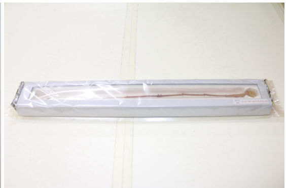
Figure 16. Sealing with oxygen-barrier film with low-humidity oxygen scavenger.
