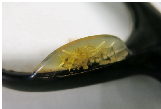
Figure 4. Nose pads of eyeglasses(51755), crack.
