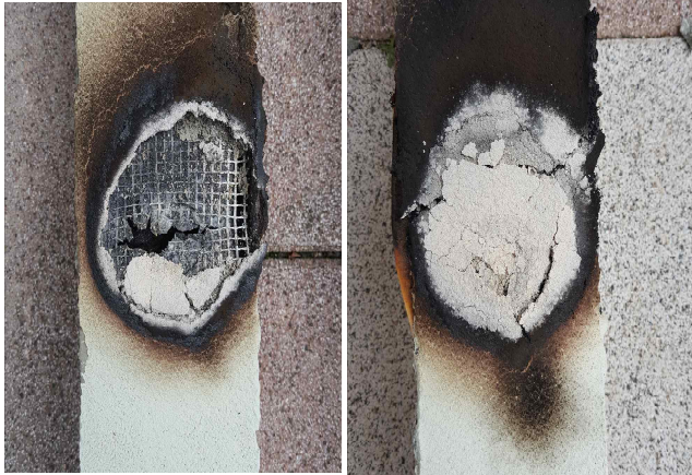
(a) Ordinary surface preparation materials (b) Surface preparation materials using expandable Graphite
