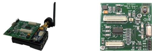
Fig. 2 Imote2 wireless sensor node platform and SHM-A sensor board
