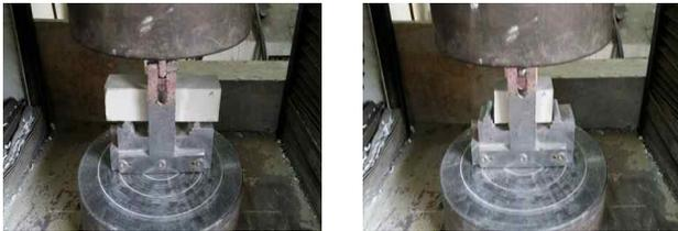
Figure 2. Flexural and compressive strength test
