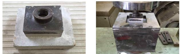
Figure 3. Bond strength test
