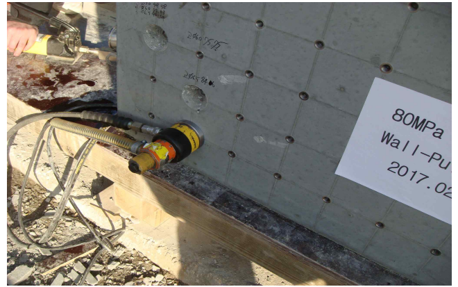
Figure 6. Pullout test for wall specimen
