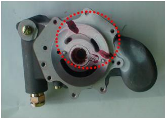
Fig. 1 The crack of the valve block on the port
