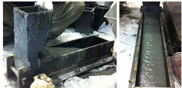
Fig. 2. Placing to Induce Shear Flow of UHPFRC in Fabricating Flexural Beam Specimen
