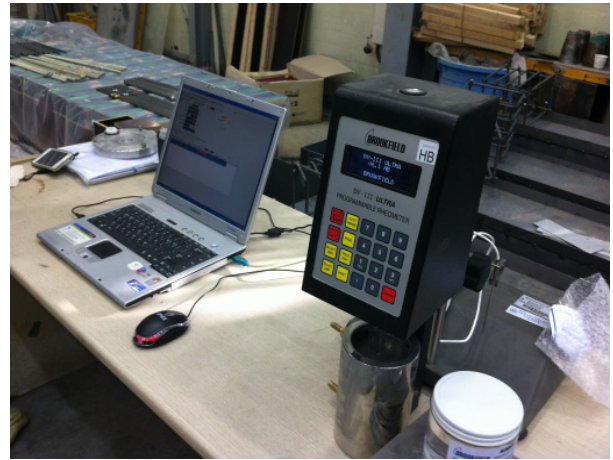
Fig. 1. Equipment for Measuring Rheological Properties
