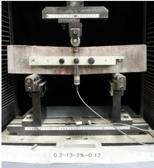
Fig. 3. Flexural Tensile Test with Notched Beam
