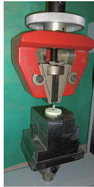
Fig. 3. Pull-out test with a cross-head speed of 0.5 mm/min in the universal testing machine.
