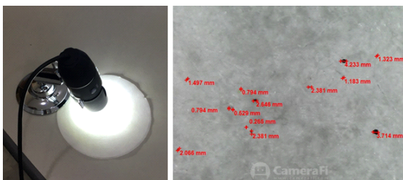
Fig. 3. Measurement of the size of pulverization matters for using Microscope.
