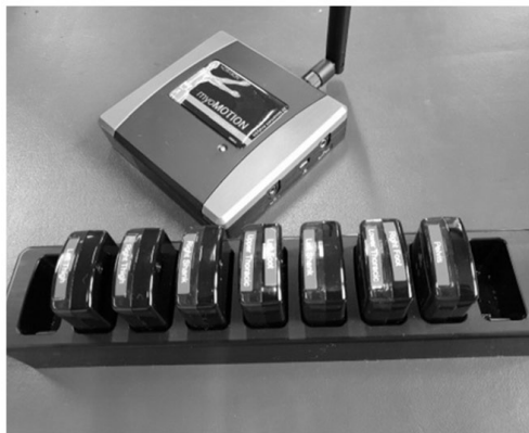
Fig. 2. 3D motion analyzer's sensor and interface
