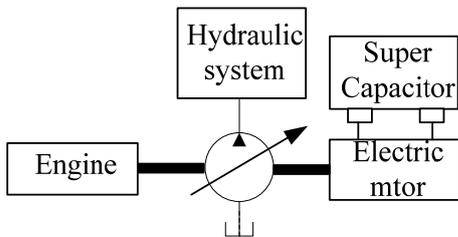
Fig. 3 The parallel hybrid hydraulic excavator research by Qing Xiao.
