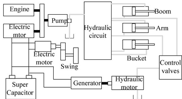
Fig. 13 ZX200 hybrid excavator of Hitachi
