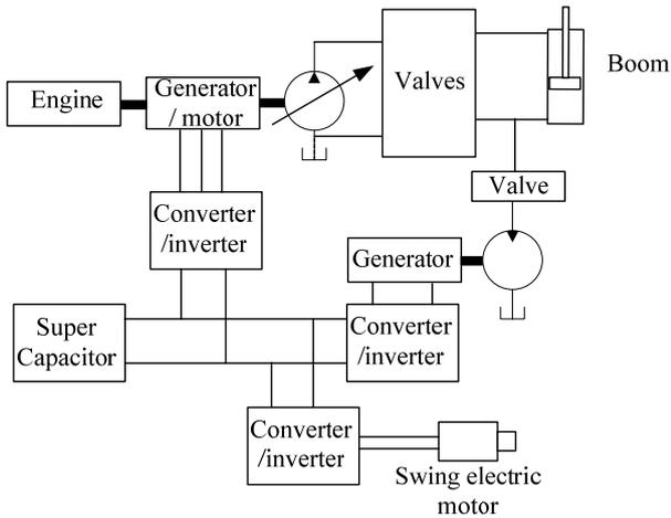
Fig. 5 The hydraulic excavator with potential energy regeneration system
