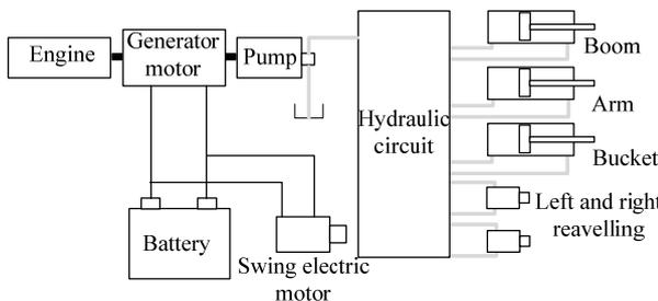
Fig. 12 The hybrid hydraulic excavator of Kobe Steel
