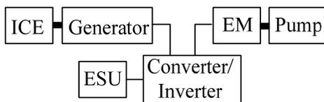
Fig. 1 Configuration of series hybrid excavator
