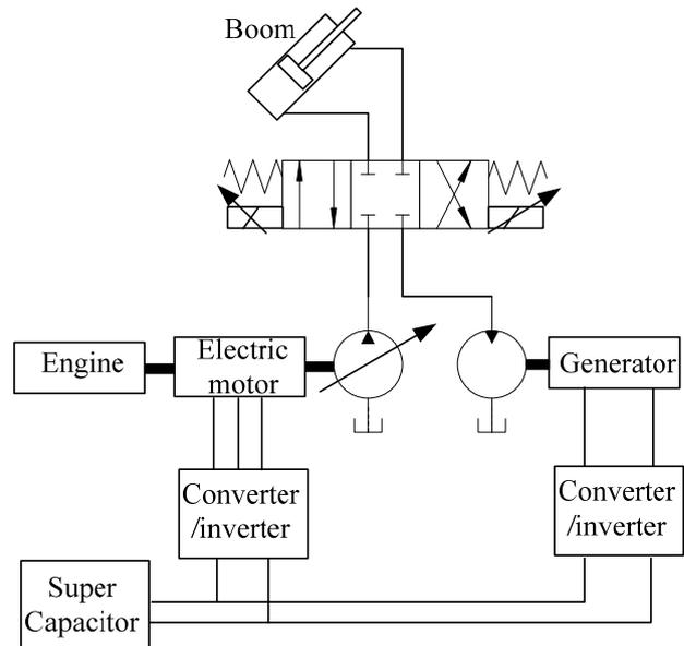
Fig. 4 Energy-saving pressure-compensated scheme for hybrid hydraulic excavators
