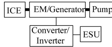
Fig. 2 Configuration of parallel hybrid excavator
