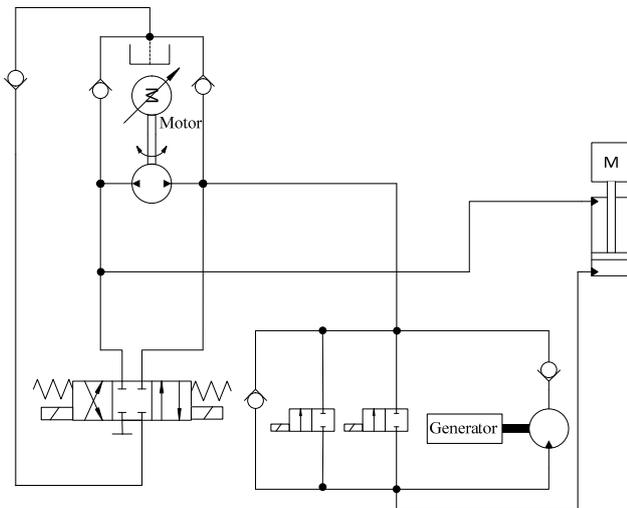
Fig. 6 One example of a hybrid hydraulic excavator
