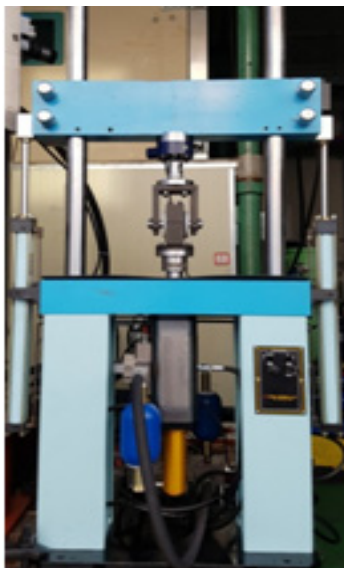
Fig. 10 Hydraulic servo actuator prototype mounting test photograph
