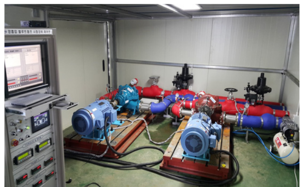
Fig. 3 Test equipment for performance and life
