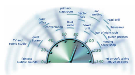
Fig. 11. Typical cases of sound pressure level [15]
