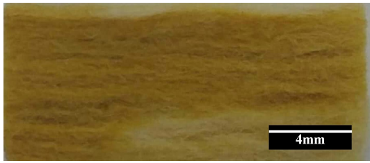
Fig. 6 Cross section of cigarette dust filtration
