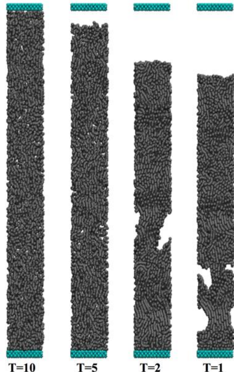
Fig. 7 Temperature-dependent cavity distributions
