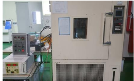
Fig. 6 Reproduction test equipments for high-temperature operation of the fuel pump
