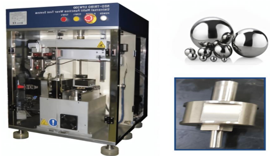
Fig. 3 Universal function wear tester & ball specimen (SUJ-2) & pin specimen (SUS440C)
