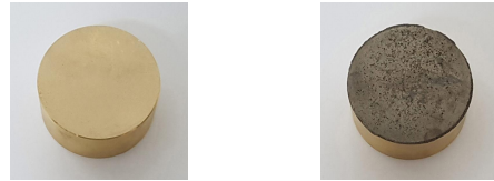
(a) Before flame spray (b) After flame spray
