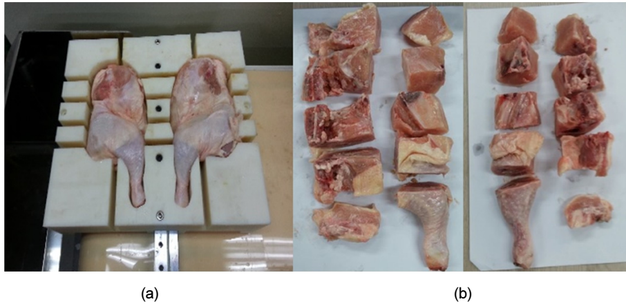
Figure 13. Chicken cutting using the automatic chicken cutting device ((a) chicken contained in a tray before cutting, (b) chicken pieces after cutting)
