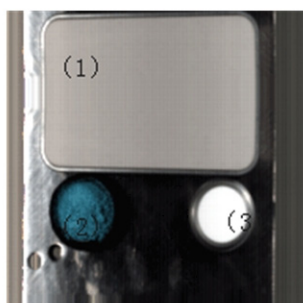
Figure 2. Image acquired by the spectral imaging spectrometer: (1) Gray board, (2) Ginseng powder, (3) White board acting as a reference.
