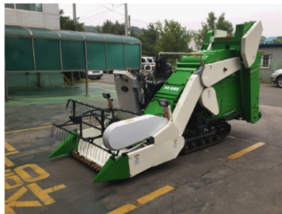
Figure 1. Photograph of the prototype small combine for harvesting miscellaneous cereal crops.
