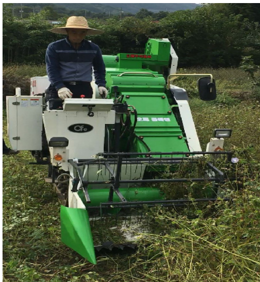
Figure 2. Photographs of the prototype small combine for harvesting buckwheat and output sample in the grain outlet.
