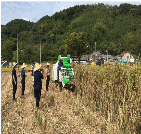
Figure 3. Photographs of the prototype small combine for harvesting adlay and output sample in the grain outlet.
