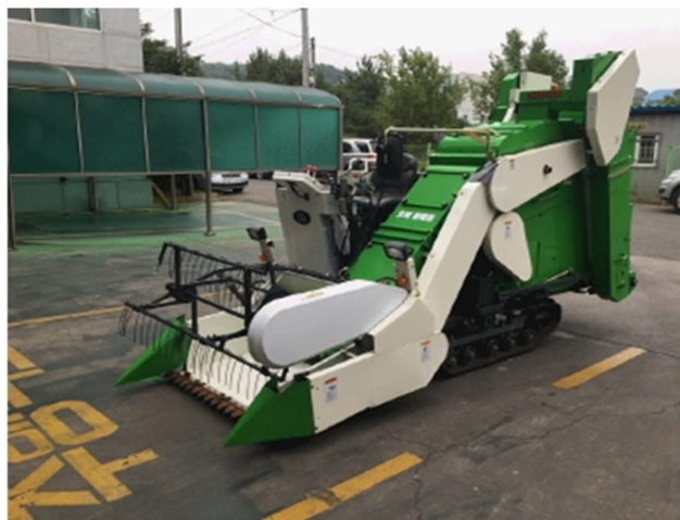
Figure 1. Photograph of the prototype small combine for harvesting miscellaneous cereal crops.
