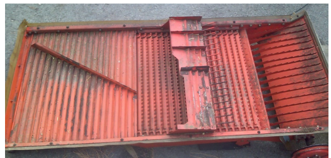
Figure 3. Shape of the sieve (cleaning shoe) of the rice combine (DSM70).
