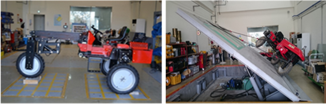
Figure 1. Views of split of weight on front and rear wheels, and static lateral stability tests.
