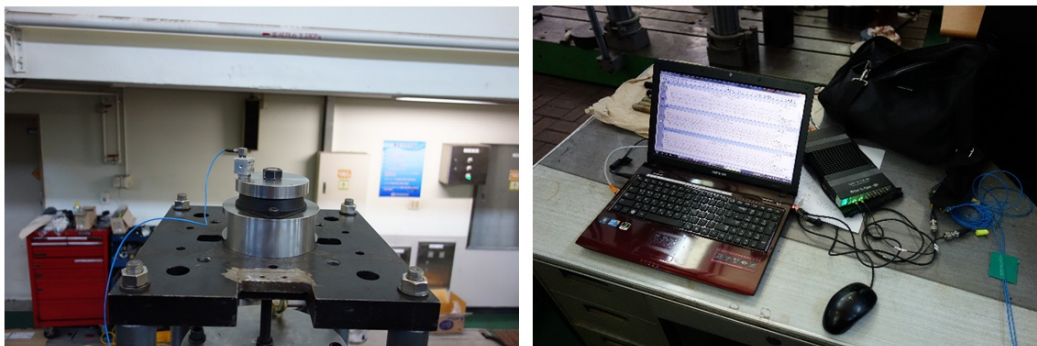
Figure 9. Accelerometer installation and signal analyzer.
