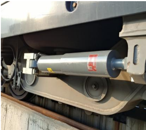
Fig. 7. Yaw damper angle adjustment
