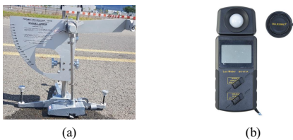
Fig. 10. Test environment measuring device (a) Skid-resistance (b) Illuminator
