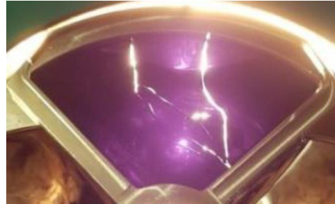
Fig. 2. The Crack of IR Transmission Filter
