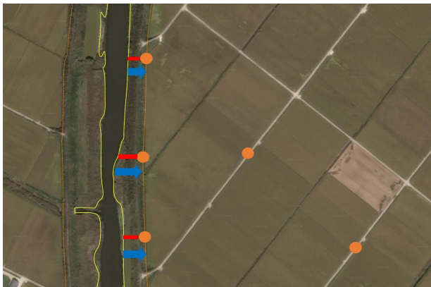
Fig. 1. Water impoundment design with river water source (yellow), water transport canals (red), and water control structures (orange). Water flow is indicated by blue arrows
