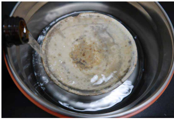
Figure 11. Reversible test with xylene.
