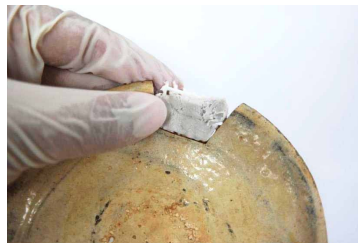
Figure 6. Gap-filling process with poly-urea putty.
