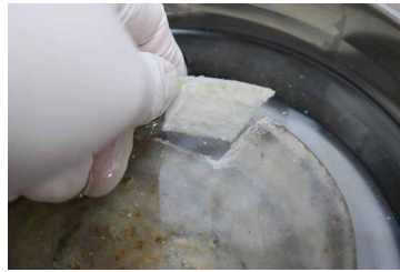
Figure 12. Separation state of restoration plate in xylene after 4 hrs.
