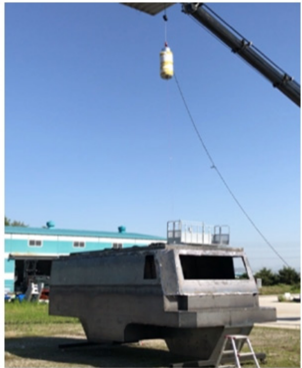
[Fig. 6] FOPS test for the body frame of the armored robot
