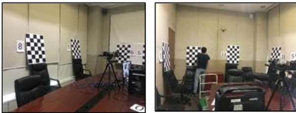
[Fig. 11] Calibration patterns for multi-camera calibration. The relative poses between patterns are not known in advance
