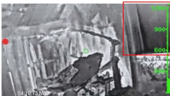
[Fig. 3] A thermal image of the indoor fire site during the flash over. It is difficult to identify the door (red box area) with thermal images only.
