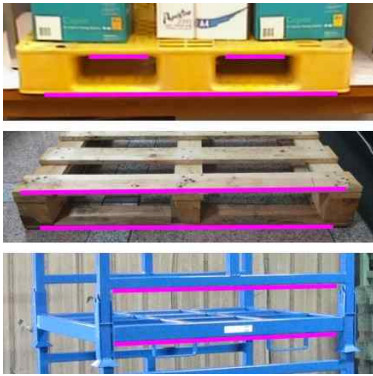
Fig. 2. Various pallet images with two or three edge lines that are useful for estimating orientation of each pallet.
