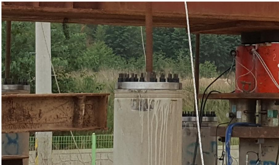
Fig. 7. Splice of reaction pile and tension steel
