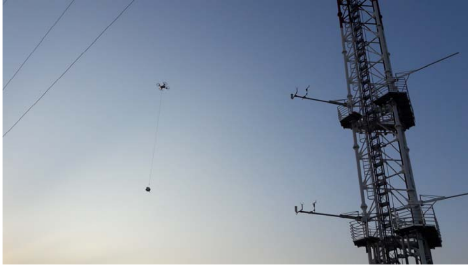
Fig. 18. Bosung Tower measurements and SSOS measurements using drone at the same height.
