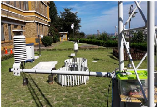
Fig. 4. Ground AWS measurement and SSOS sensors measurement at the same height.
