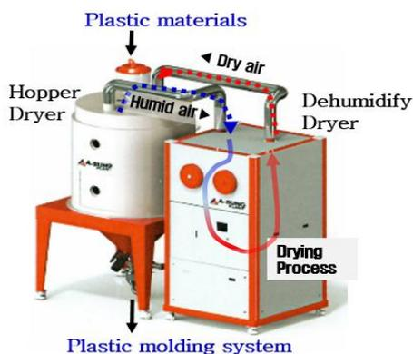
Fig. 1. Dehumidify Dryer in Plastic Molding System
