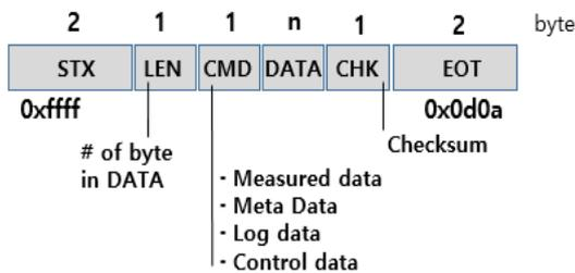
Fig. 5. Data format between dryer and interface module
