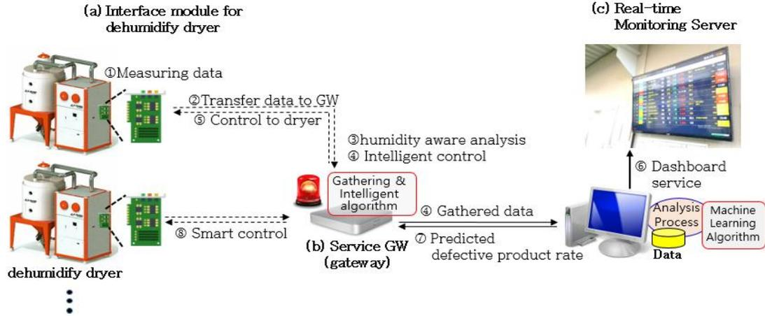
Fig. 2. Smart Factory System Model for Plastic Molding System
