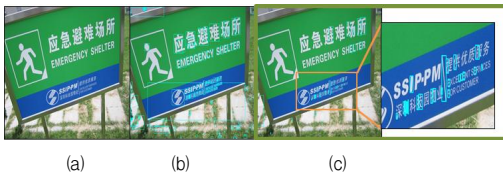
Fig. 10. Incorrect removal non-text results using aspect ratio. (a) Original Image (b) Comparison area (c) Result of Labeling.
