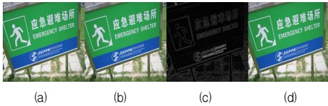
Fig. 6. Boundary contrast enhancement results using unsharp mask. (a) Original Image (b) Blur image (c) Detected Boundary (d) Contrast enhancement of object boundaries.
