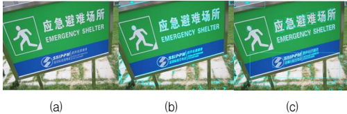
Fig. 9. Results of MSER region labeling (a) Original Image (b) Result of Contour Labeling (c) Result of rectangle Labeling
