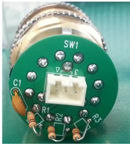
Fig. 2. The explosion proof type's switch
