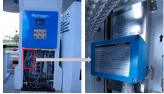
Fig. 1. Location of mass flow meter in dispenser (MFM)
