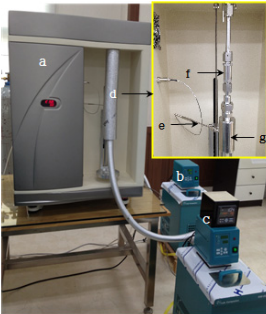
Fig. 3. Thermal Analysis apparatus for low temperature hydrogen storage alloy (a) main P-C-T apparatus, (b) thermostatic circulator for internal temperature control, (c) thermostatic circulator for reactor temperature control, (d) a reaction vessel for a low temperature, (e) RTD temperature sensor, (f) Inline filter, (g) reaction vessel for a low temperature
