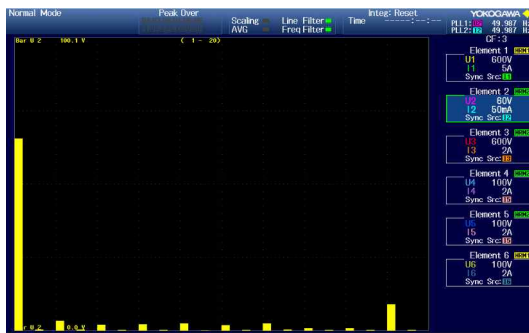
Fig. 29. Voltage THD measured using THD meter
