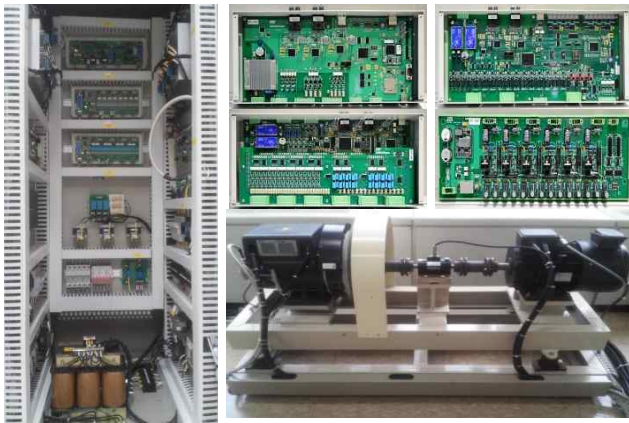
Fig. 17. Prototype of the 5kVA LCI system and MG-set
