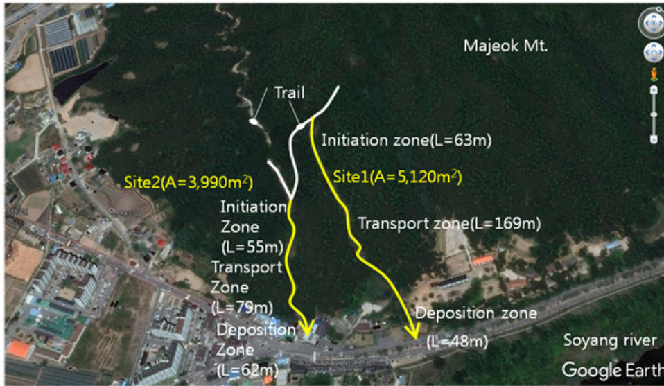
Fig. 1. Site detail of chunjeon-ri landslide
