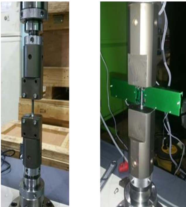
Fig. 4 Tensile test, conducted with the initially designed jig and specimen
