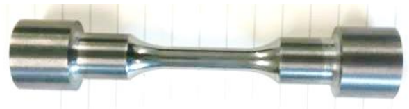
Fig. 3 Initially designed WC-Co alloy tensile specimen
