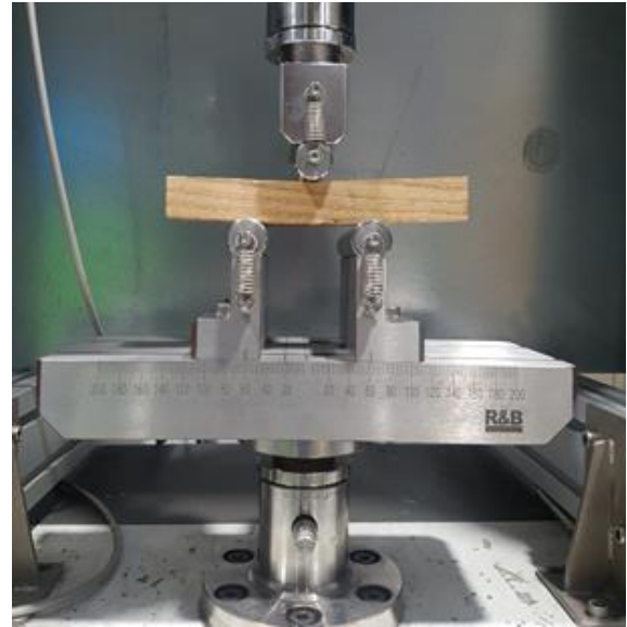
Fig. 8 3-point bending test of wood specimens
