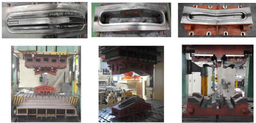
Fig. 8 Shape of the tool sets for fabricating prototypes
