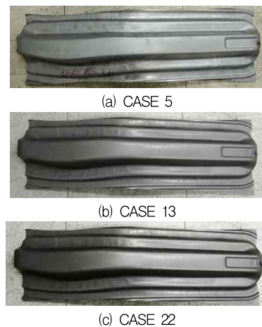
Fig. 14 Shape of the prototype obtained from the experiment with the variable blank holding force
