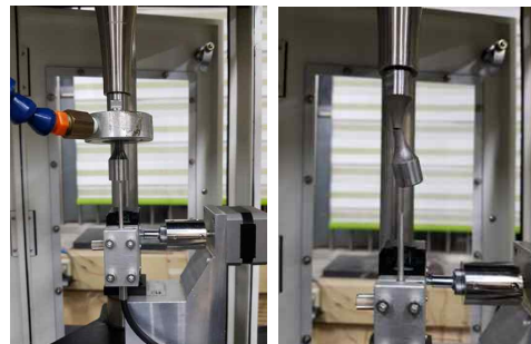
Fig. 6 Ultrasonic fatigue test (left side is during test, right side is after fracture)
