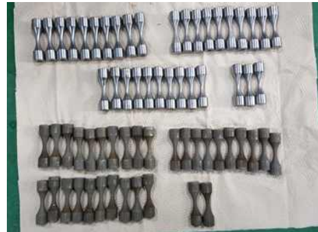
Fig. 5 Ultrasonic fatigue test specimen (upper surface polished, lower surface laser sintered)
