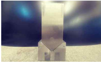
Fig. 9 Punch and die for restriking
