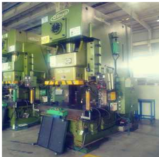
Fig. 5 The 200-ton force press used in the experiment
