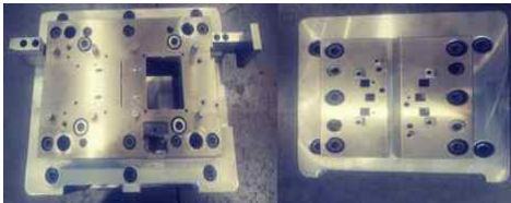
Fig. 4 Photo of assembled die
