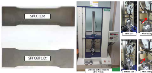
Fig. 8 Specimen & system for tensile test
