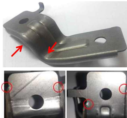
Fig. 10 Problems in process(crack)
