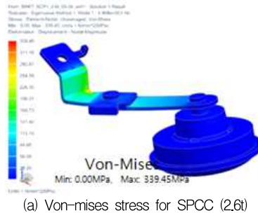
(a) Von-mises stress for SPCC (2.6t)
